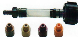
57-11-1 Tip kit for lean dilution ratios 750:1, 1000:1, 1500:1, 2000:1 Includes 4 metering tips, 8 ft. 1/4" vinyl hose and 1/4"x3/8" barb adapter
